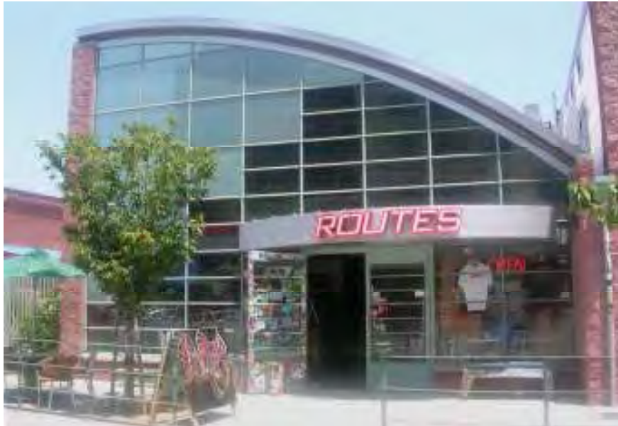
Guidelines 15 and 3 Example. This business uses a modest sign in conjunction with a unique building design to attract attention. As well, it illustrates how storefronts can provide visual interest through transparency and three-dimensional variations in the façade.
